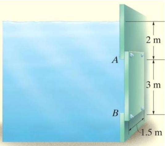
Determine the magnitude and location of the resultant hydrostatic force acting on the submerged rectangular plate AB. The plate has width 1.5m. The density of the water is  $1000 \text{ kg/m}^3$
