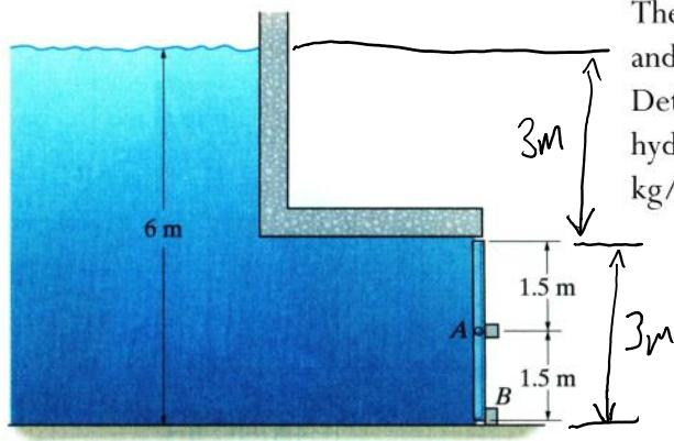
The 2m wide rectangular gate is pinned at its center A and is prevented from rotating by the block at B. Determine the reactions at these supports due to hydrostatic pressure. The density of the water is 1000 kg/m<sup>3</sup>
