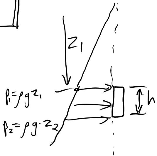
$$F_2 = \overrightarrow{\text{Area}} \cdot \overline{h} = \underbrace{\overrightarrow{\text{Area}} \cdot \overline{h}}_{p_1} + \underbrace{\overrightarrow{\text{Area}} \cdot \overline{h}}_{p_2 - p_1}$$
