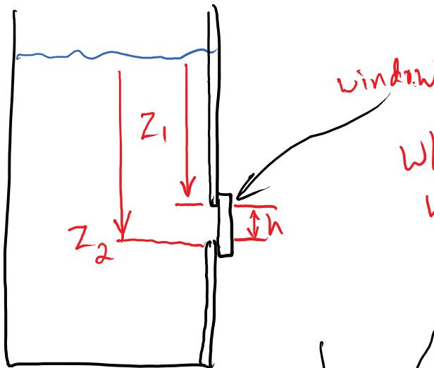
What force acts on the window? (suppose the window has a width  $w$ )
