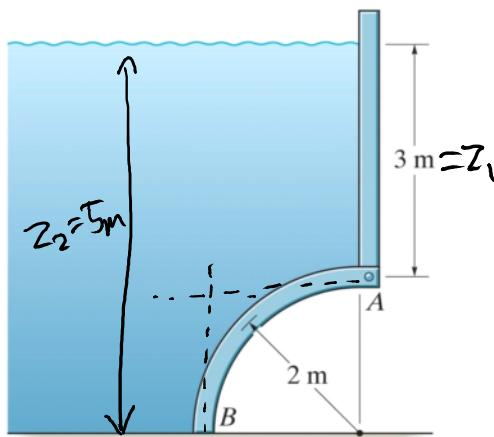
The arched surface AB is shaped in the form of a quarter circle. If it is 8 m long, determine the horizontal and vertical components of the resultant force caused by the water acting on the surface. The density of the water is 1 Mg/m<sup>3</sup>
